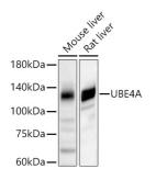
Western blot analysis of various lysates, using Anti-Ube4a Antibody (A11638) at 1:3,000 dilution. The secondary antibody was Goat Anti-Rabbit IgG H&L Antibody (HRP) at 1:10,000 dilution. Lysates/proteins were present at 25µg per lane. The blocking buffer used was 3% non-fat dry milk in TBST. Detection was with a ECL Basic Kit. Exposure time: 60s.
