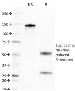
SDS-PAGE analysis of Anti-BCMA Antibody [BCMA/2366] under non-reduced and reduced conditions; showing intact IgG and intact heavy and light chains, respectively. SDS-PAGE analysis confirms the integrity and purity of the antibody.
