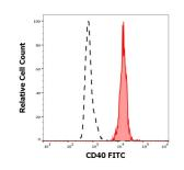
Separation of human CD40 positive lymphocytes (red-filled) from neutrophil granulocytes (black-dashed) in flow cytometry analysis (surface staining) of human peripheral whole blood stained with Anti-CD40 Antibody [HI40a] (FITC) (20  $\mu$ l reagent / 100  $\mu$ l of peripheral whole blood).
