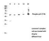
Western blot analysis of customer's using Anti-p53 (phospho Thr18) Antibody.
