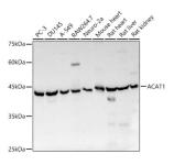
Western blot analysis of various lysates, using Anti-ACAT1 Antibody (A89814) at 1:1,000 dilution. The secondary antibody was Goat Anti-Rabbit IgG H&L Antibody (HRP) at 1:10,000 dilution. Lysates/proteins were present at 25µg per lane. The blocking buffer used was 3% non-fat dry milk in TBST. Detection was with a ECL Basic Kit. Exposure time: 10s.
