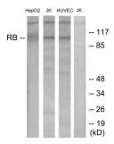
Western blot analysis of lysates from HepG Jurkat, and HUVEC cells using Anti-Retinoblastoma Antibody. The right hand lane represents a negative control, where the antibody is blocked by the immunising peptide.
