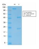
SDS-PAGE analysis of Anti-MMP9 Antibody [rMMP9/1769] under non-reduced and reduced conditions; showing intact IgG and intact heavy and light chains, respectively. SDS-PAGE analysis confirms the integrity and purity of the antibody.
