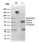
SDS-PAGE analysis of Anti-TDRKH Antibody [PCRP-TDRKH-1H2] under non-reduced and reduced conditions; showing intact IgG and intact heavy and light chains, respectively. SDS-PAGE analysis confirms the integrity and purity of the antibody.
